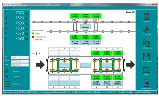
Our intuitive, multilingual ptwX software is designed and developed in-house and provides real time 'live' displays. Multiple customisations such as weighing units and information on weight differentials are also available
