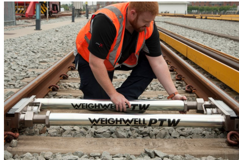
4. Positioning the PTW into the track.
