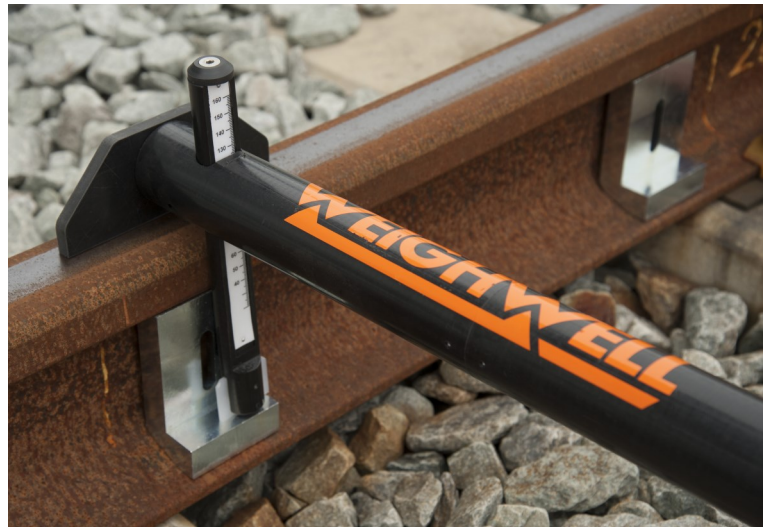
2. Select location and check rail head wear.
