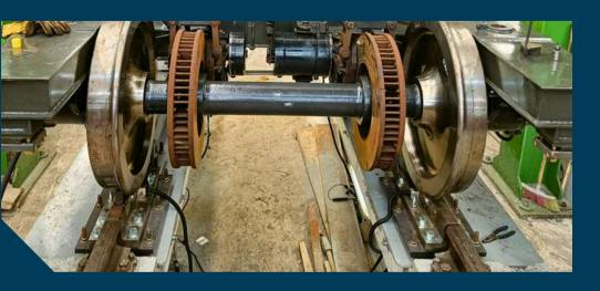
Installed within existing infrastructure, the Bogie Workshop System replaces sections of rail with high-precision loadcells (TrackCells).
