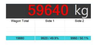
WiM Software Designed for the in-motion weighing of rail vehicles. It can visually highlight imbalanced loads
