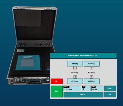
The Static Weighing Indicator features a touchscreen interface with an integrated QWERTY alphanumeric keypad. It displays wheel weights for up to four axles (eight wheels) and provides weighing results in kilograms (10kg increments).
