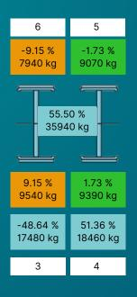
Designed for static weighing, this software captures the weights based upon your rolling stock configuration. The main features are adjustable tolerances for error conditions and wheel numbering specific to your rail vehicle.
